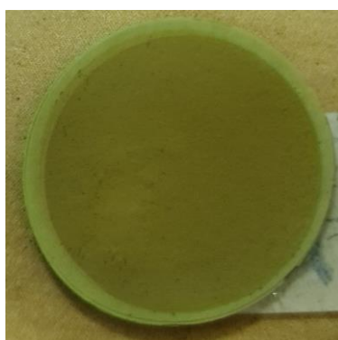
Figure B.10. Anode disc after sputter deposition of electrolyte layer on its surface.
