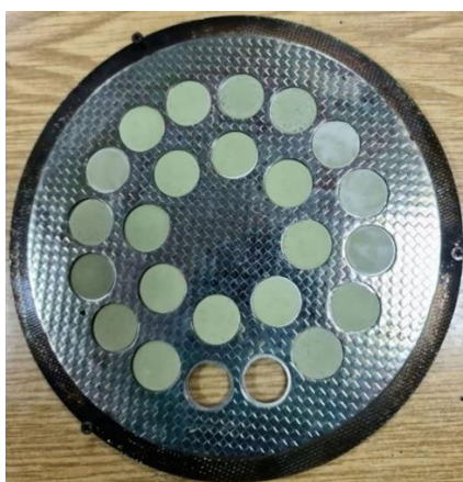
Figure B.8. Placed anode layer after preparing by tape casting method on sample holder to do sputter deposition on them.
