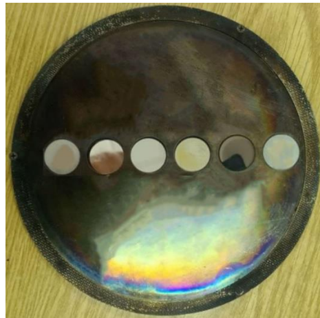
Figure 3.3. Sample holder used for sputter deposition of cathode materials.
