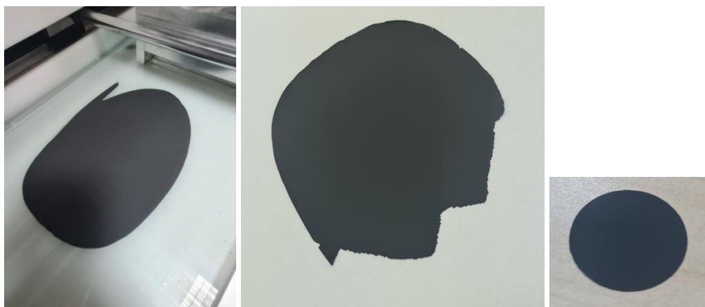
Figure B.5. Dried anodes fabricated via tape casting.
