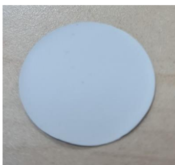
Figure B.3. Dried single electrolyte layer produced by tape casting technique.
