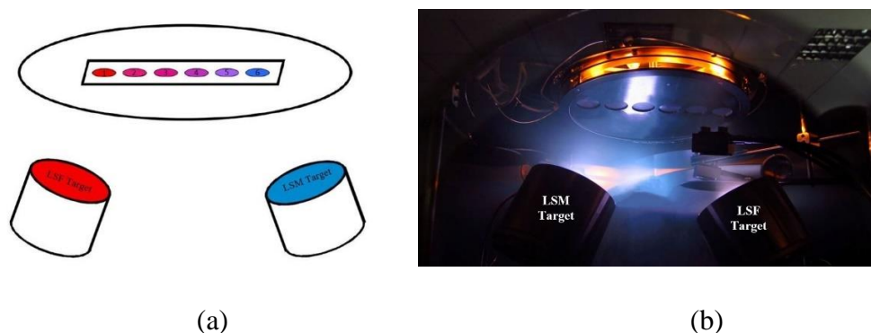
Figure 3.4. (a) Schematic representation of combinatorial deposition (b) View from the vacuum chamber with combinatorial deposition.
