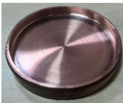
Figure A.1. Copper holder used as a casing for sputter targets.
